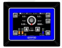
The **DOSIFOR™** - **5NPI** control unit consists of a high luminance, sunlight readable 7" color touch screen display that is easy to use filled with useful information for the user. This unit displays actual water and foam concentrate flow rates, as well as totalizers and foam concentrate pump operating information.
